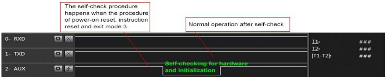
Timing Sequence Diagram of AUX when self-check
